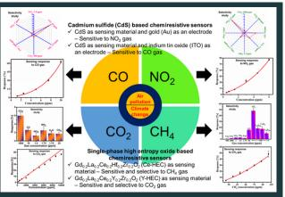
Figure 1. Summary of the gas sensing performance of the fabricated sensors for monitoring two types of gases.
